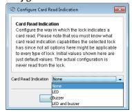
Different locks can have a different mechanism for audio-visual indication of successful credential reading. Here it is possible to disable credential read indication or to set it to LED. Some Aperio locks have support for other mechanisms such as buzzers.
