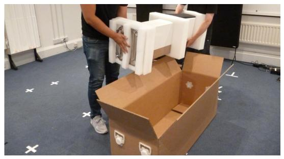
7. Push foam base against metal base to keep in position and gently place product into cardboard packaging. Ensure speaker is face up.
