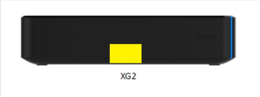
Samsung XG2 – Manufacturer model # SX022ANM/SX022ANC. IR target indicated in yellow. This model has 1 RF In, 1 RF Out, Analog Audio (RCA L & R) Out, Composite Video Out, HDMI Out, SPDIF Out.
