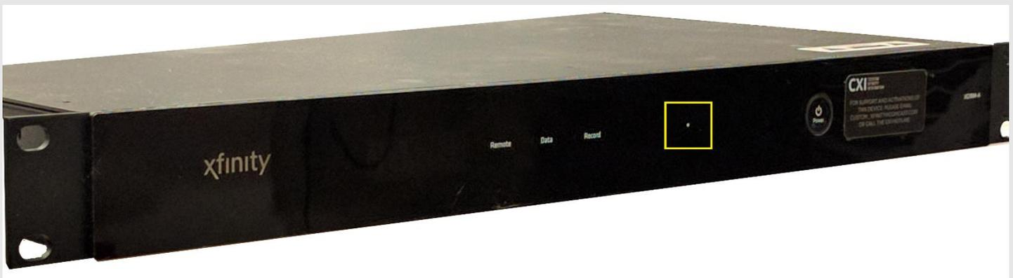
Arris XG1v1 – Manufacturer model # AX11RANM/AX11RANC. IR target indicated with white dot in the center of the yellow box outline. This model has 1 RF In, 1 RF Out, 1 HDMI Out, Analog Audio (RCA L & R) Out, SPDIF Out.
