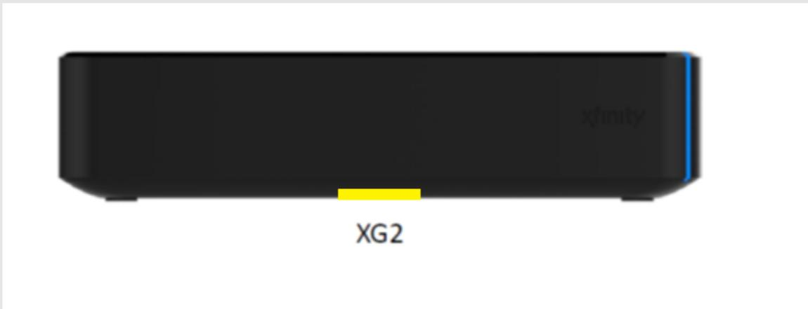
Pace XG2 – Manufacturer model # PX022ANM/PX022ANC. IR target indicated in yellow. This model has 1 RF In, 1 RF Out, Analog Audio (RCA L & R) Out, Composite Video Out, HDMI Out, SPDIF Out.
