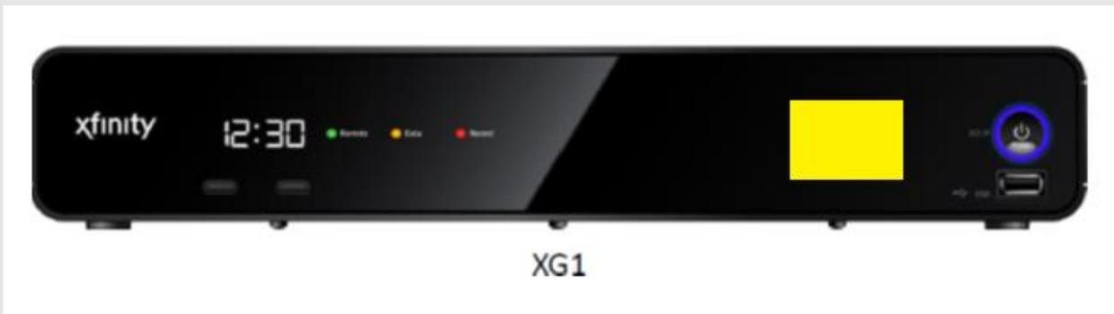
Arris XG1v3 – Manufacturer model # AX013ANM/AX013ANC. IR target indicated in yellow. This model has 1 RF In, 1 RF Out, Analog Audio (RCA L & R) Out, Composite Video Out, HDMI Out, SPDIF Out.
