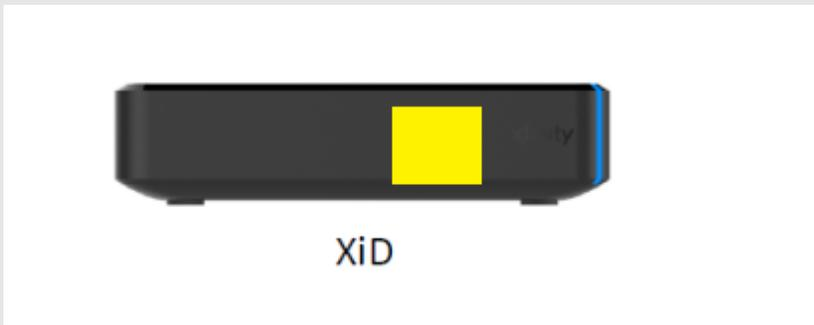
Pace XiD – Manufacturer model # PXD01ANI. IR target indicated in yellow. This model has one RF input, one RF output and one HDMI output.
